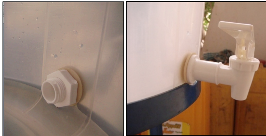
Figure 6-4: Left, Jam nut and washer, which attach the Tomlinson Industries spigot to the inside of the Kosim safe storage container; Right, Tomlinson Industries spigot and washer attached to the outside of the Kosim safe storage container.
