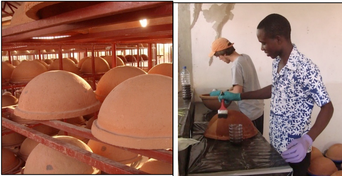
Figure 1-2: Left, Hemispheric ceramic water filters on cooling racks after firing process at PHW; Right, PHW employee and MIT graduate student painting filters with colloidal silver solution
