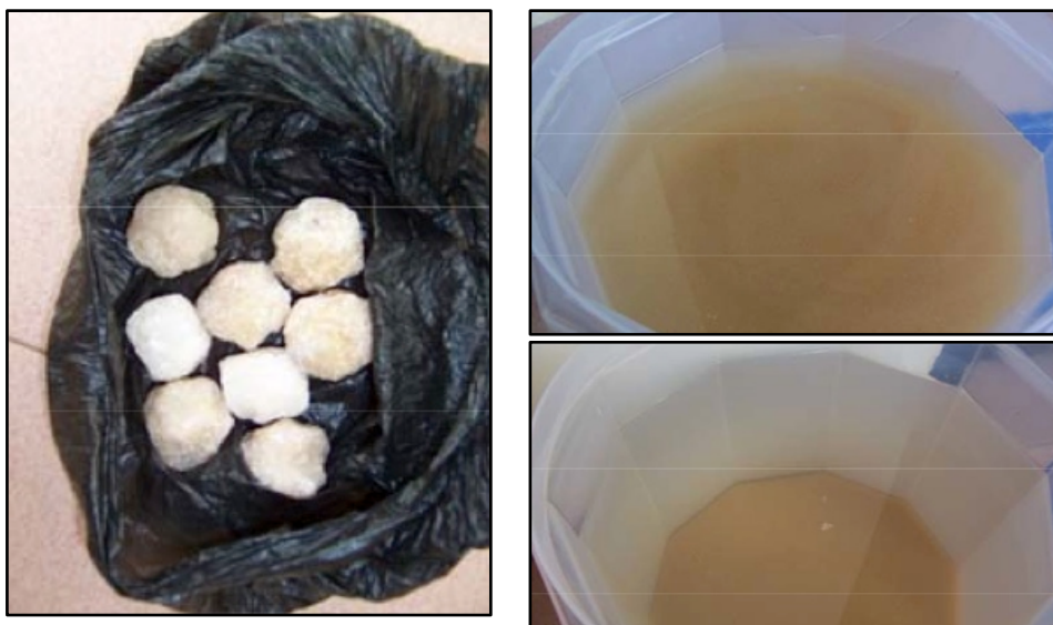
Figure 4-9: Right, alum balls (Credit: Melinda Foran); Left top, water being treated with alum (Credit: Melinda Foran); Left bottom, Water after treatment with alum (Credit: Melinda Foran)
