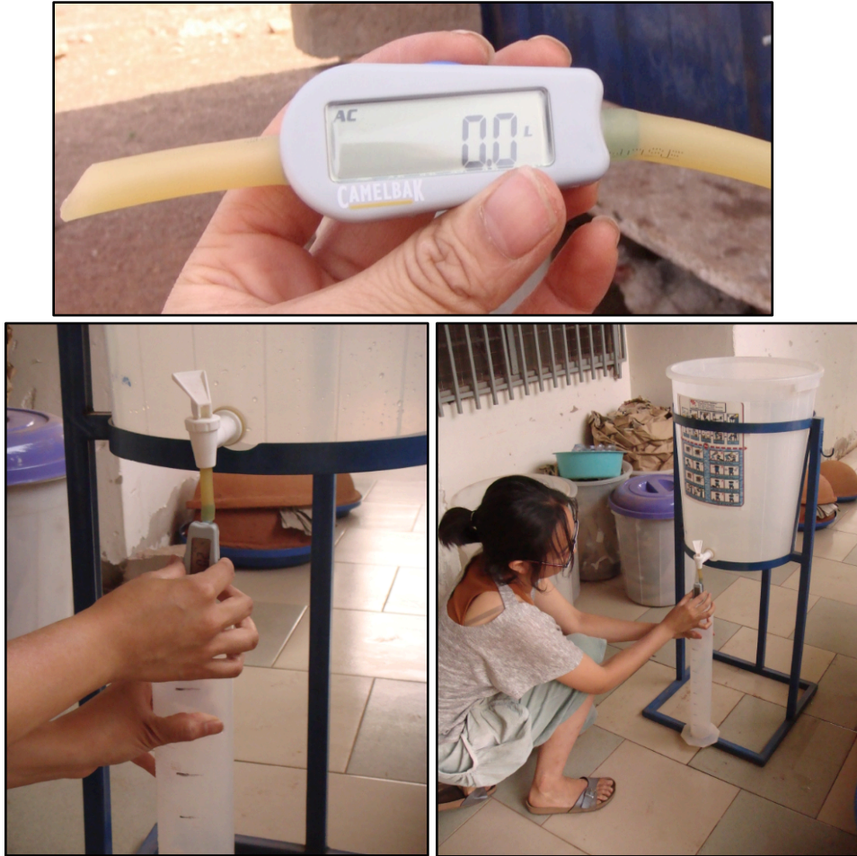
Figure 6-3: Top, Flow Meter™ plugged into flexible plastic tubing; Bottom, experimental set-up and close-up of experimental set-up (Credit: Jonathan Thibault).
