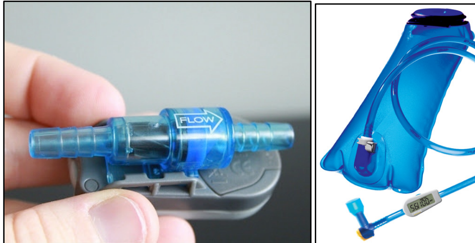
Figure 6-1: Left, Camelbak® Flow Meter™ (Credit: http://www.scalerchelis.com/ ); Right, intended use of Camelbak® Flow Meter™ is to measure personal hydration during exercise by gaging flow from Camelbak® hydration packs (Credit: http://gearjunkie.com/ ).
